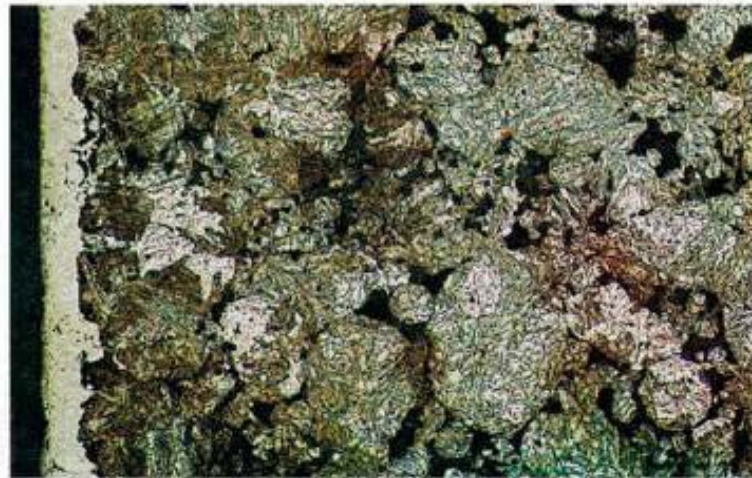
Fig. 10.15 Section of an induction-hardened chain sprocket. (Distaloy AB + 0.7 wt.% C, density 7.1 g/cm 3 ). The l
