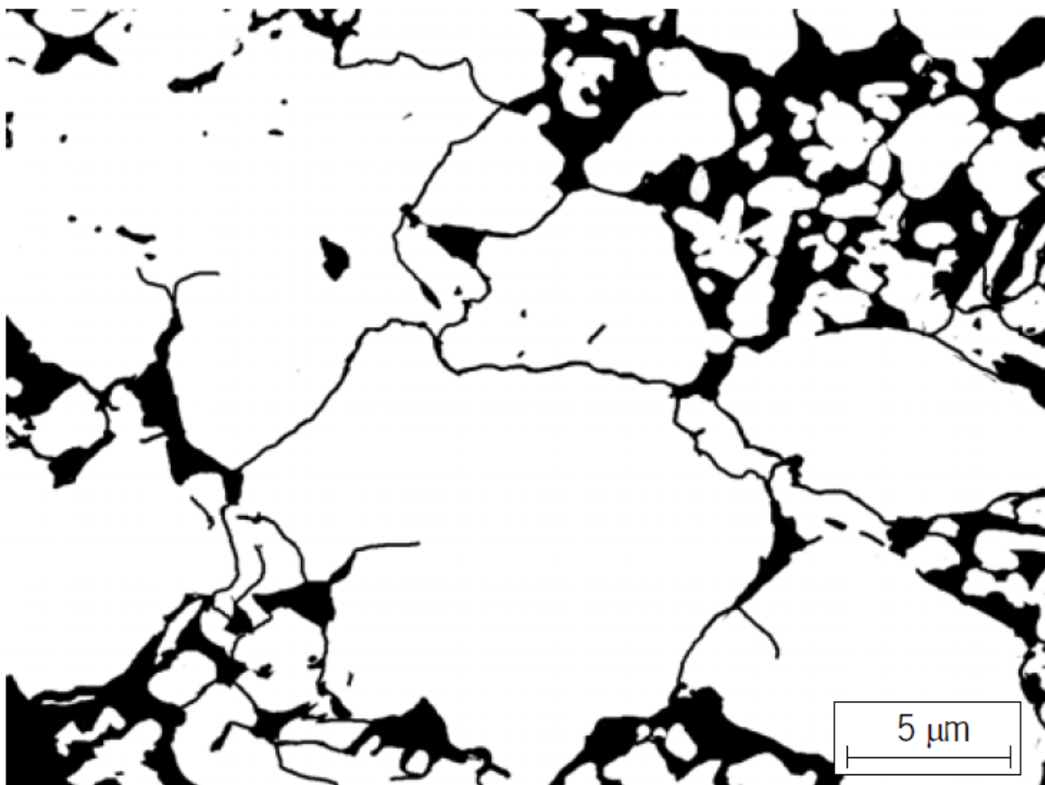
Figure. 4.3. Adaptation of surface contours due to plastic deformation of adjacent powder particles. Electrolytic copper powder compacted at 200 \text{ N/mm}^2 . [4.4]
