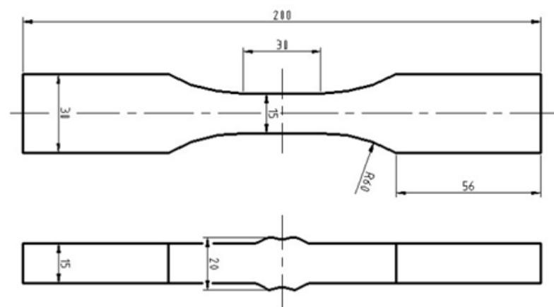
Figure 6. Shape and geometry of the HCF test specimens for butt welded joints (BWJ).
