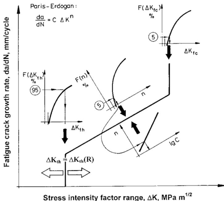
Figure 9. The previously proposed method for determination of fatigue crack propagation limit curves [25].
