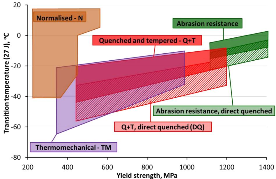
*Figure 2. Combination of strength and toughness typical for commercial steels [15][16][18][30].*
