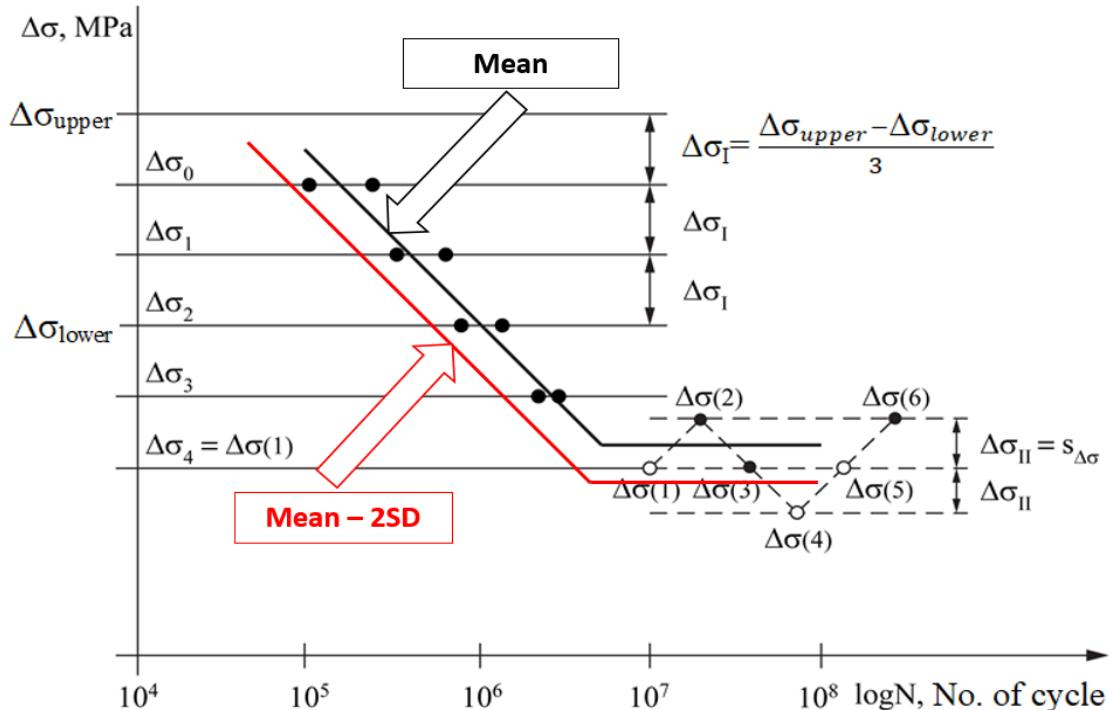
Figure 7. Determination of high cycle fatigue strength curves, „Mean-2SD” S-N curves.
