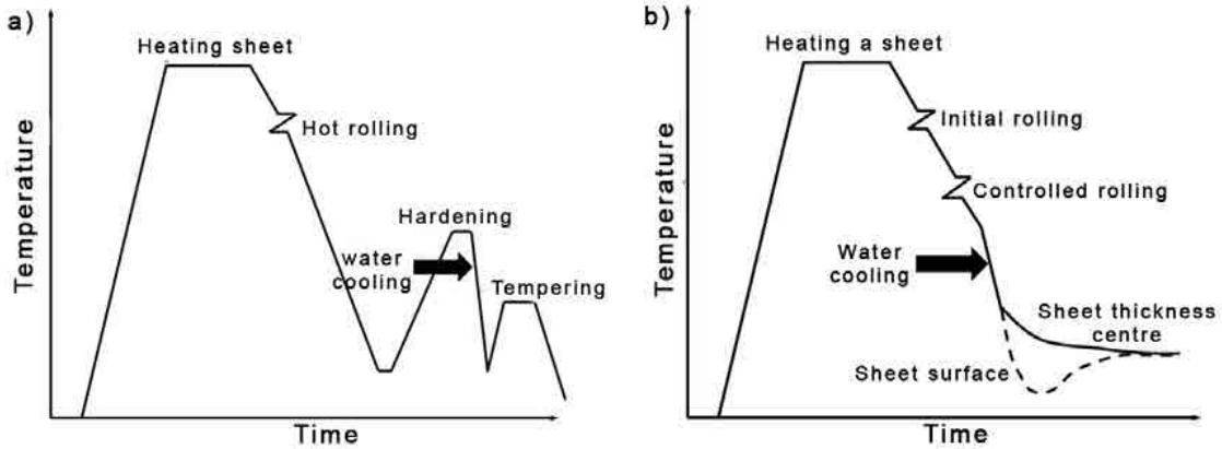
*Figure 3. Diagrams of production processes of toughened steels a) hardening and tempering processes, b) direct hardening process [16].*
