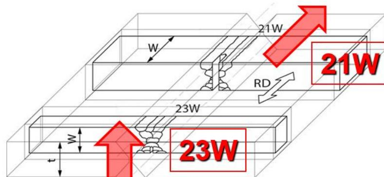
Figure 5. TPB specimen locations in welded joint with notch directions (RD = rolling direction).
