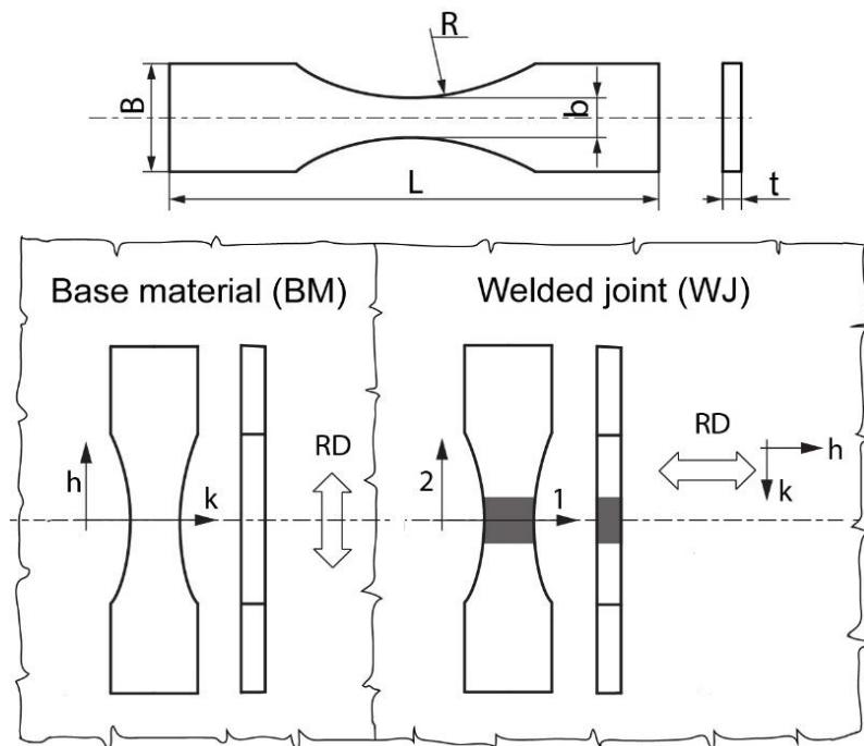
Figure 4. The geometry, the location and the designation of the HCF test specimens for base materials (BM) and welded joints (WJ).
