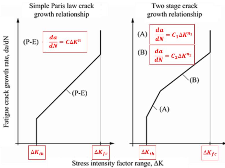
Figure 8. Simple and two-stage fatigue crack growth relationships, based on [3].
