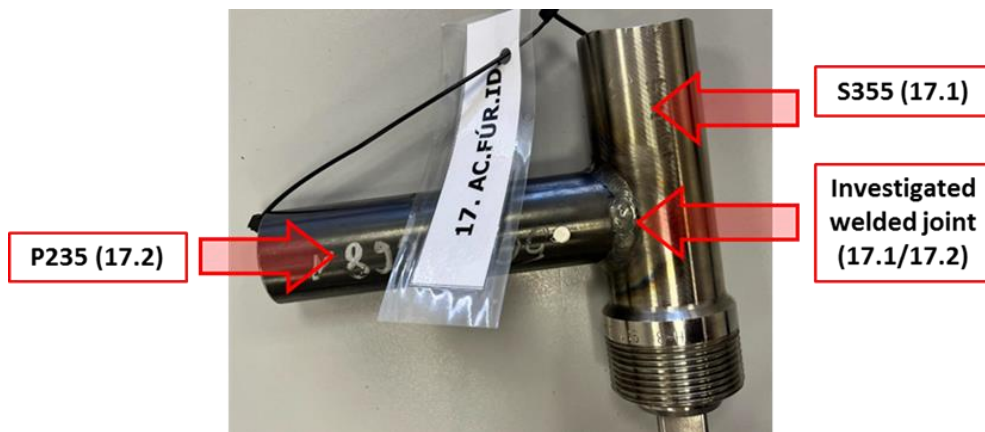
Figure 11. The NA50 welded hot tap fitting (17) made from two different steel grades.
