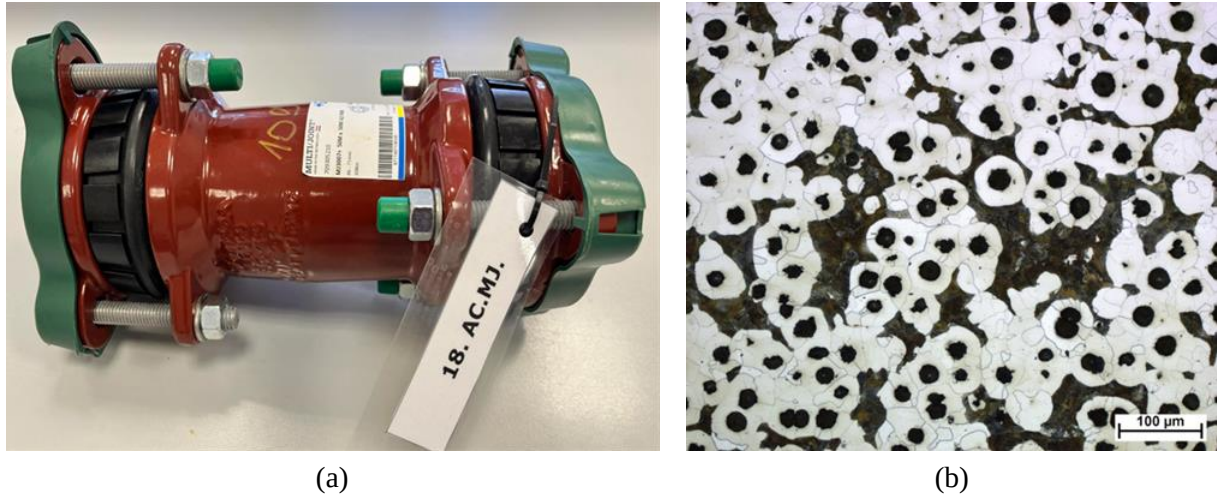
Figure 16. The structure of the Multi/Joint connection system (a) and the microstructure of the brick-red cast iron body (b) etched with 3% \text{HNO}_3 , N=200\times .
